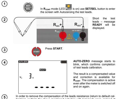
In order to remove the compensation of the leads resistance (return to default calibration), perform the above-mentioned activities with test leads open, instead of test results, the display will show message **oFF** (compensation of test leads is turned off).
