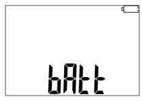
The battery pack is fully discharged, all measurements are blocked. The meter switches off automatically after 5 sec.
