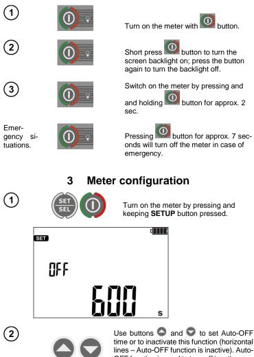
time or to inactivate this function (horizontal lines - Auto-OFF function is inactive). Auto-OFF function is used to turn-off inactive meter after a preselected time.
