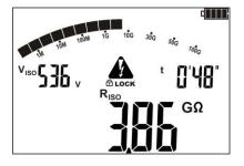
View of the screen during measurement. **IDCCK** means that the measurement was started with ENTER button or by pressing and holding START button for approx. 5 sec.
